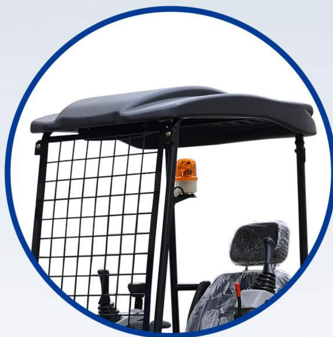
Top protection against falling objects
